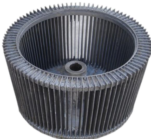
Based on the physical model of classification in vaned rotors, the fundamental difference between the exclusive use of a forced vortex flow (i.e. classification at the outer edge of the vanes) and the combined use of forced vortex/free vortex flow (i.e. classification in the interior vane free area) is derived.
